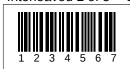
Interleaved 2 of 5 + CHECKSUM
